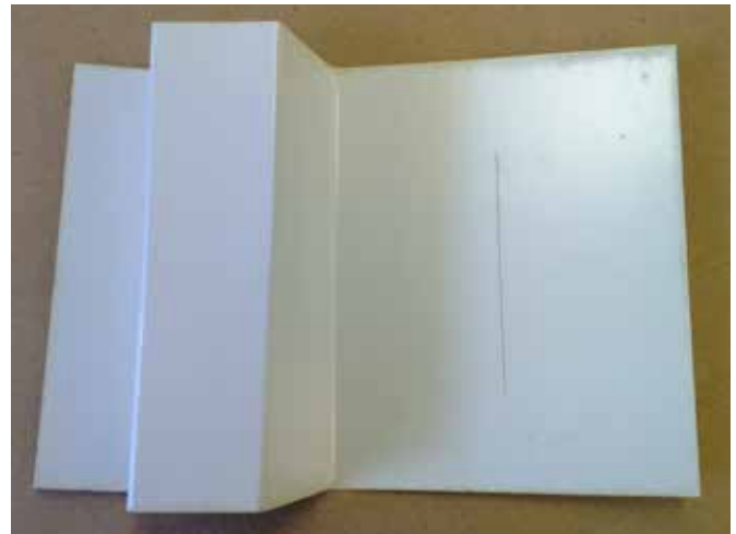
Figure 11: PMY0500FP Primer with Silicone Polyester Topcoat
