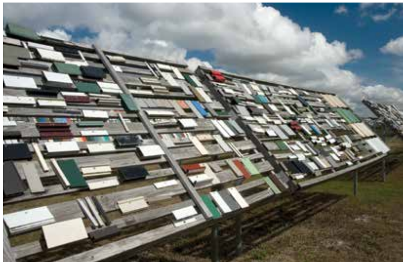
Figure 1: Fort Myers exposure site with thousands of test panels.
