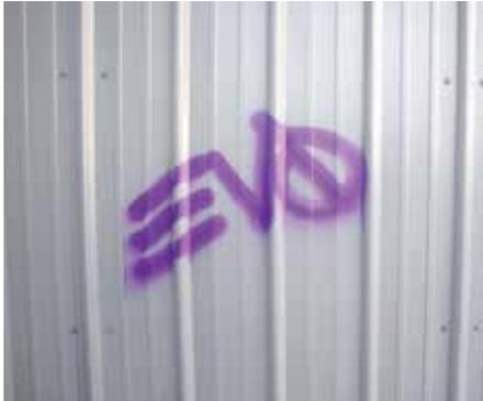
BEFORE: Spray paint graffiti markings on surface coated with Sherwin-Williams Coil Coatings’ ASTM-compliant coating.
